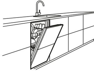
**02** Locate the dishwasher close to the water supply and drain pipes. Having the dishwasher close to the sink makes loading easier and avoids spills on the floor.
