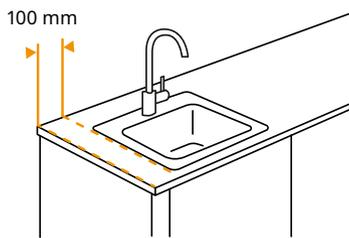
**01** Use a small sink that fits into a 600 mm cabinet. Make sure to have at least 100 mm between the sink and the edges of the worktop to make the construction sturdy.
