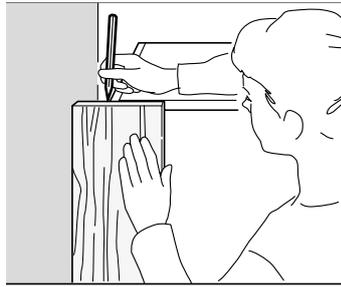
Place the newly cut edge of the filler piece against the wall (it should fit perfectly). Mark the edge of the cabinet on the top and bottom of the filler piece. Draw a straight line from these points and cut.
