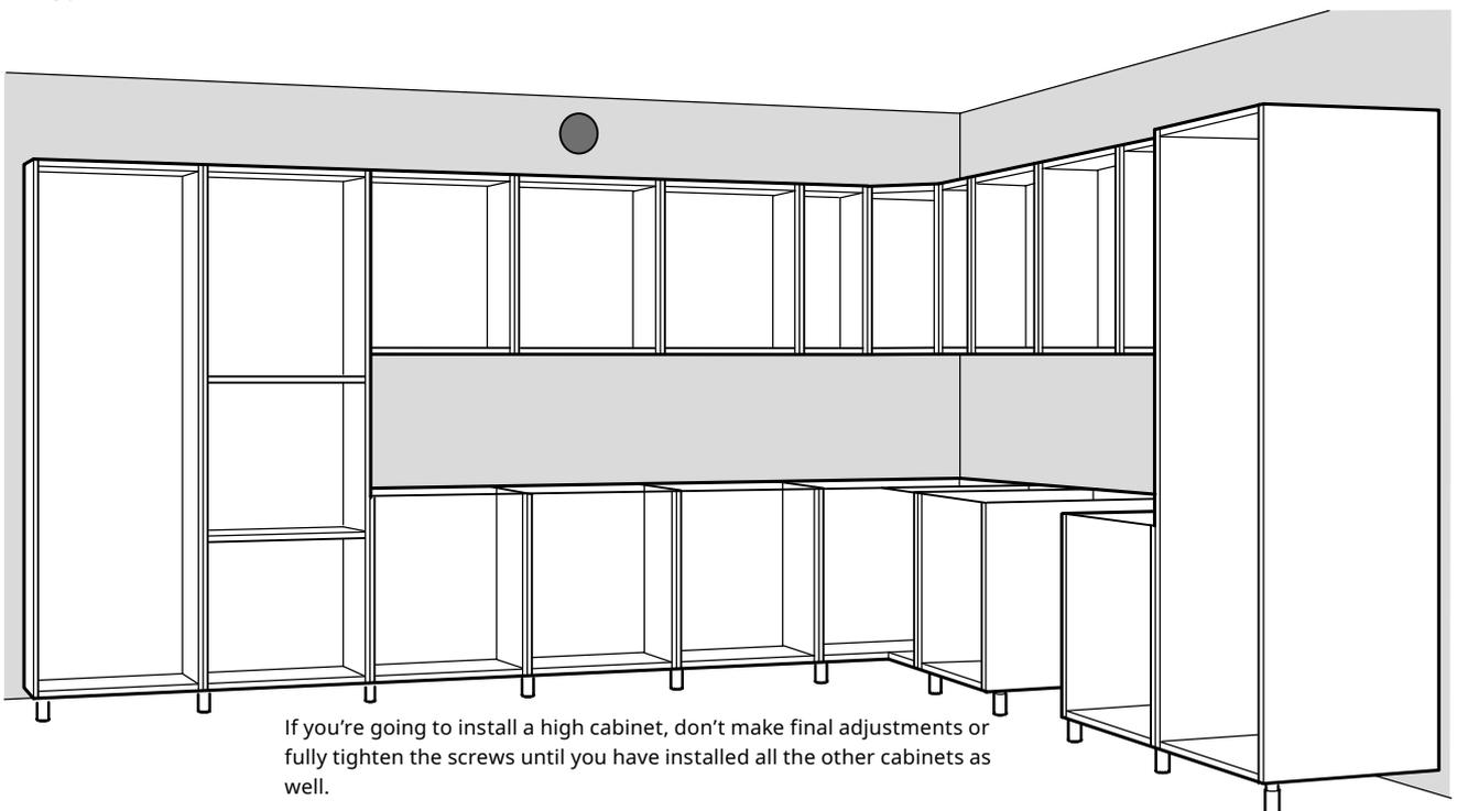
If you're going to install a high cabinet, don't make final adjustments or fully tighten the screws until you have installed all the other cabinets as well.
