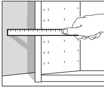
Check the wall with your spirit level to see if it is straight. If the wall is even, measure between the wall and the cabinet and mark this distance at the top and bottom of the filler piece.
