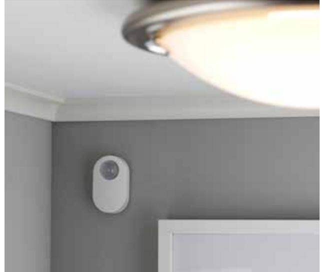
Set the motion sensor for day or night mode. Day mode is always motion-activated; night mode is only motion-activated when it’s dark. Adjust the time setting to turn off the light source after 1, 5 or 10 minutes.
