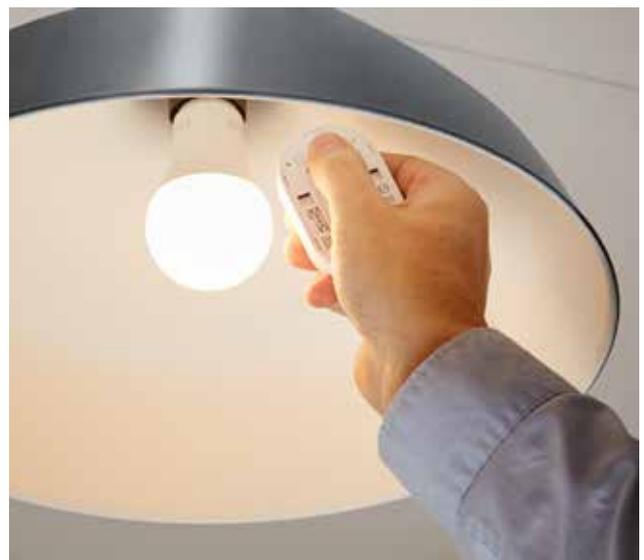
If you want to add more light sources to the motion sensor, hold the motion sensor close to the light source (no more than 5 cm away). Press and hold the pairing button for at least 10 seconds and you see a red light on the motion sensor. Your light source will start to dim and flash to indicate it’s been successfully paired.
